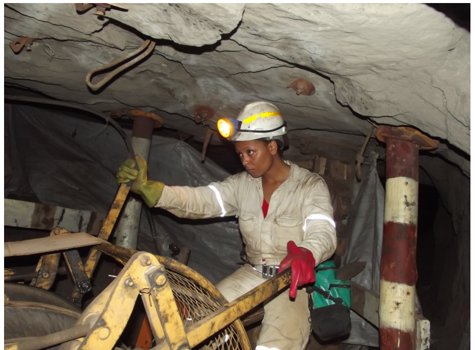
Asanda operating a scraper winch underground. A winch pulls ore from the blasted face to the tip. [Photograph: Provided]
