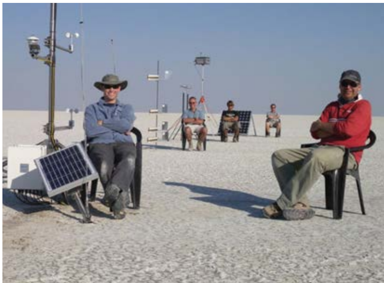
One of the eleven observation sites on the Makgadikgadi Pan in Botswana. The sampling equipment measures wind and dust as well as surface conditions and processes.
